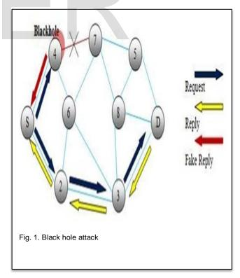
AODV is an On Demand routing protocol which has two phases as Route discovery and Route error [3]. If the source desires to communicate with destination to send the packet, it checks the existing routing table
